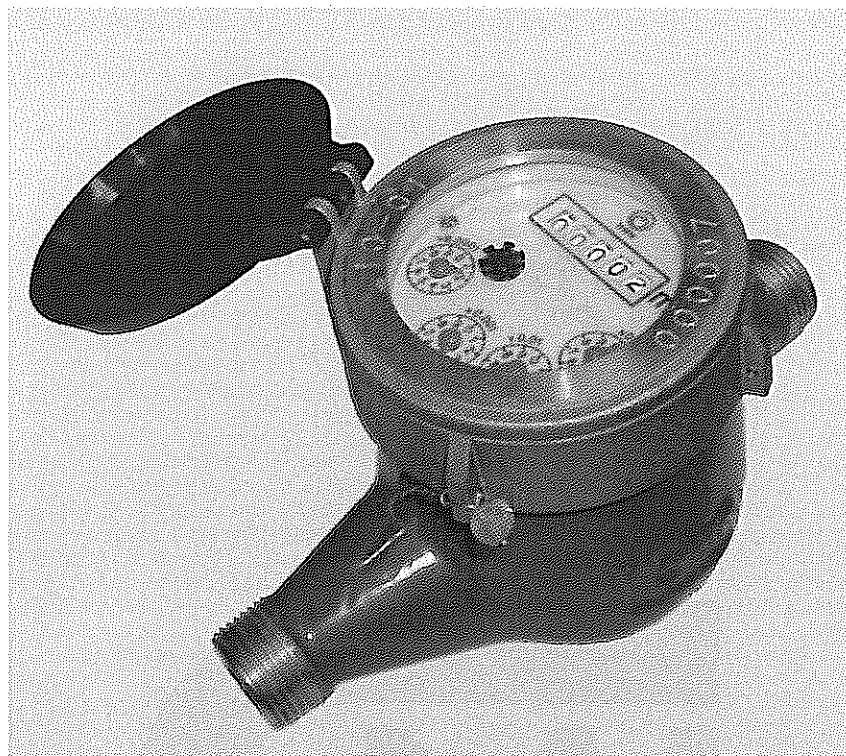
Figure 14: The sealing of the water meter type PD-SDC (E4):
